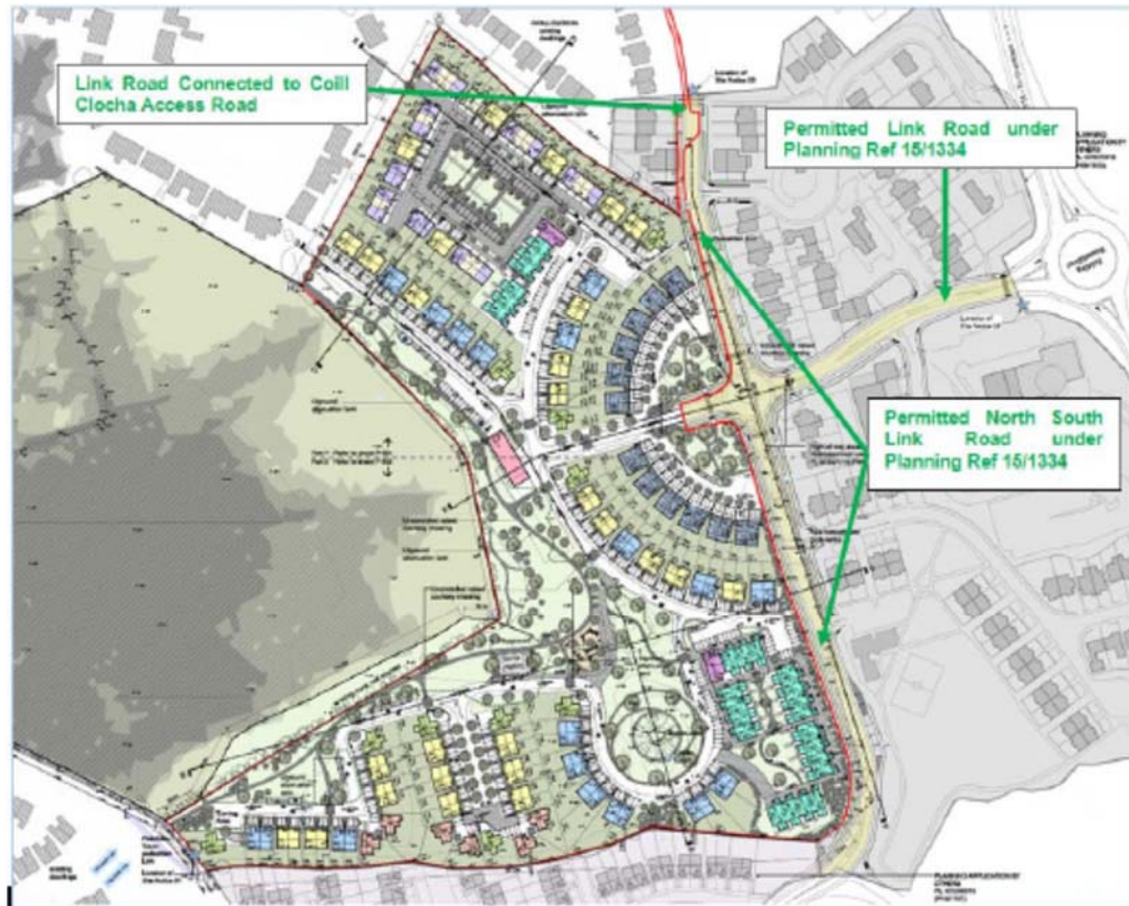
Figure 3.1: Proposed Development in context of Road Network Infrastructure Permitted under GCC PR 09/1925; ABP Ref 07.237219 & 15/1334. Image extracted from Figure 2.2 of Traffic and Transportation Statement
